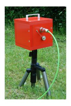
Only one SHFT-02e is required to measure the magnetic field variations in 3 orthogonal axis. The sensors and its electronics are enclosed in a shock resistant plastic case. The SHFT-02e is connected to the metronix *ADU-07* data logger (or any other custom electronics) by a cable of up to 10 m length. The high quality of the *SHFT-02e* data is achieved by a unique design for the ultra low noise preamplifier.
